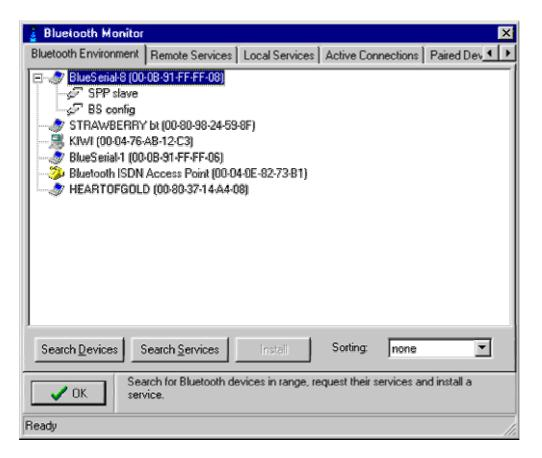
Install a virtual serial port on the "BS config" service from your Bluetooth application. Please consult the documentation of your Bluetooth PC application how this is done. Then you can start the configuration software on this port. You can do this either from the command line with
